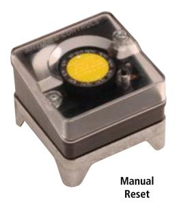
The Versa Plus gas pressure switch accurately monitors pressure and breaks the electrical control when pressure rises above or drops below the desired setpoint. It is made with a durable plastic enclosure and has a diecast aluminum inlet base.
